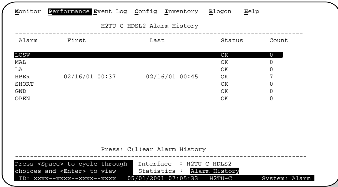
Figure 24. H2TU-C HDSL2 Alarm History Screen
