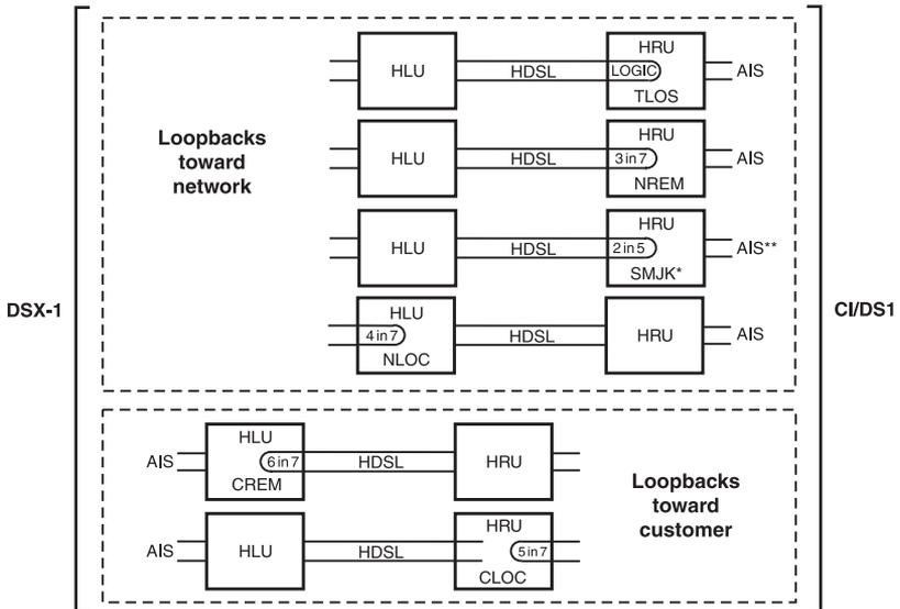
\* The Smart-Jack loopback is a metallic loopback in the HRU Lists 6 and 7. It is a logic loopback in HRU Lists 1 through 5.
