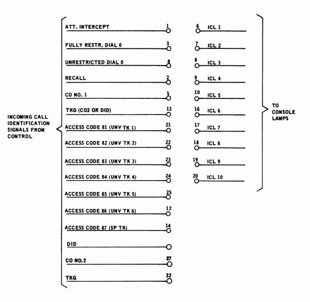
Note: Pin 26 or 27 is strapped to Pin 32 when assigning TKG (Pin 13) to an ICL.
