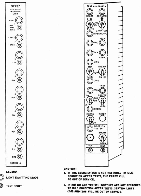
Fig. 3 – QPJ97-Type Circuit Pack **Maintenance Test Unit**
