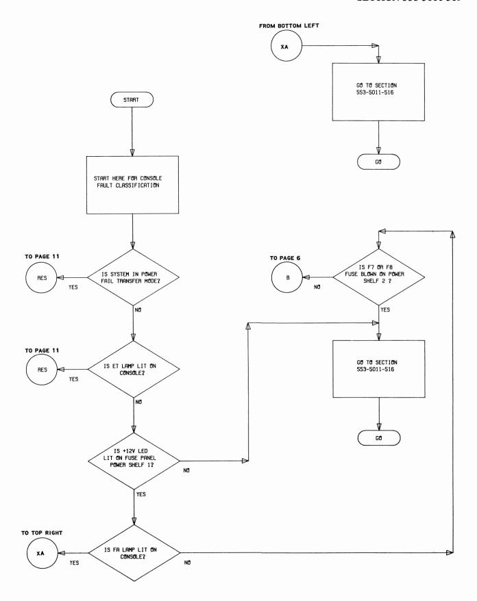
Flowchart 1 — Console and Traffic Measurement Fault Classification
