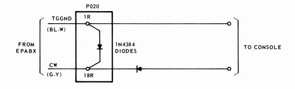
Fig. 2(b) - Call-Waiting Audible Signal Connections
