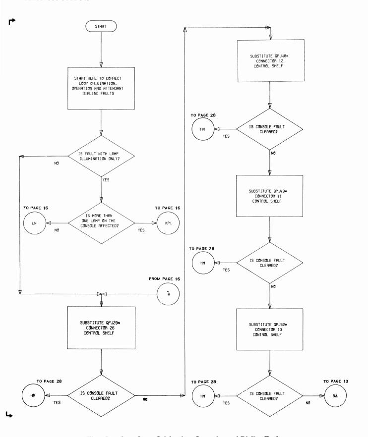
Flowchart 2 - Loop Origination, Operating and Dialing Faults
