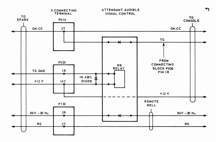
Fig. 2(a) - Extension of Console Audible Signal
