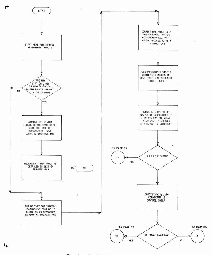
Flowchart 8 - Traffic Measurement Faults
