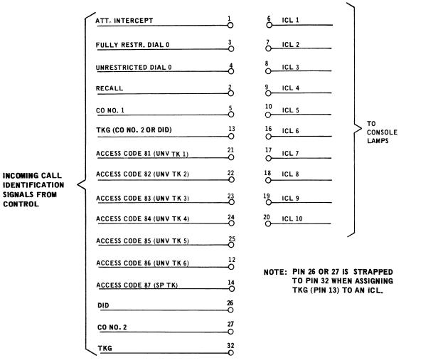
Fig. 1 – I/C Call Identification Signals and Lamps – Pin Designations on TB4 Strapping Block (Control Shelf)
