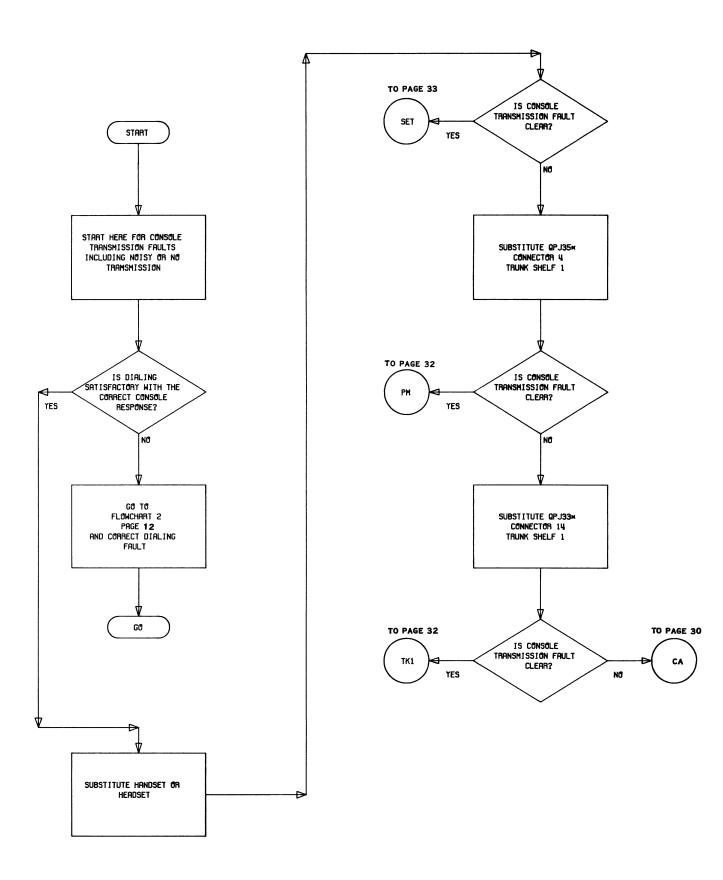
Flowchart 3 - Console Transmission Faults
