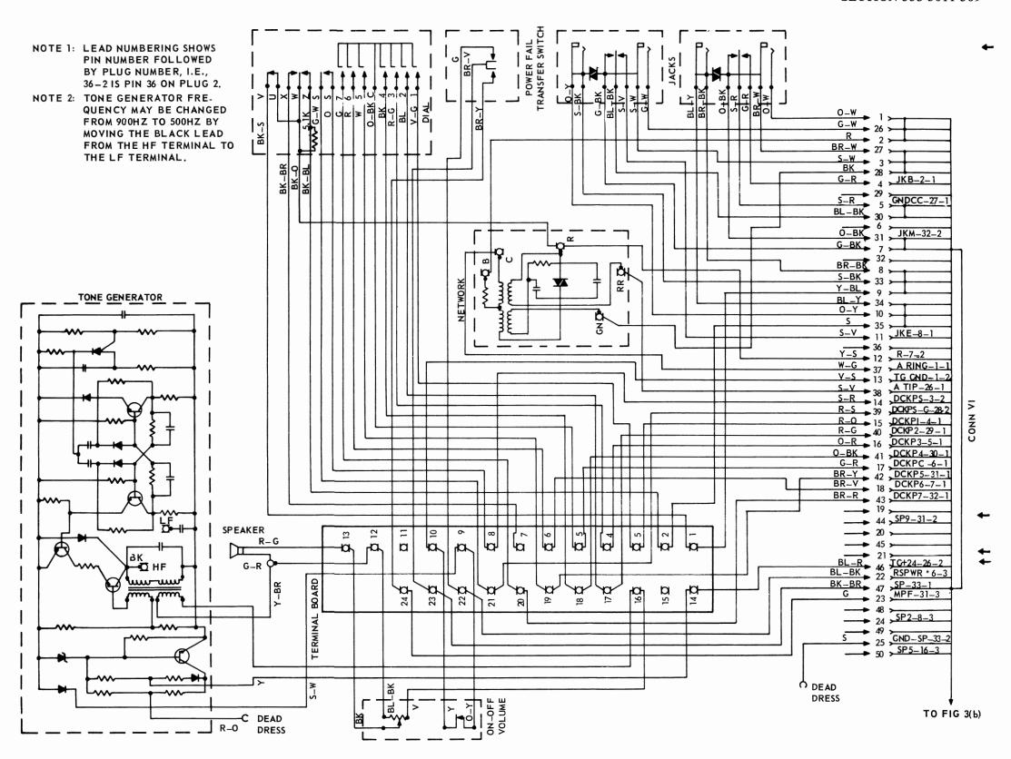
Fig. 3(a) — Attendant Telephone Wiring Diagram for QCN100B and QCN102A Consoles
