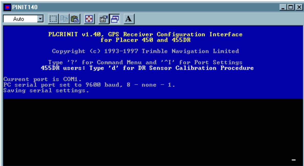
For ease of reading the rest of the screen representations, they will be shown as boxed text. The main calibration menu is shown below. The odometer calibration must precede the gyro calibration. The Backup light installation may be verified at any time.
